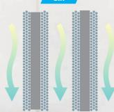
The fan operation after shut down helps dry water droplets to keep the coils dry and clean
